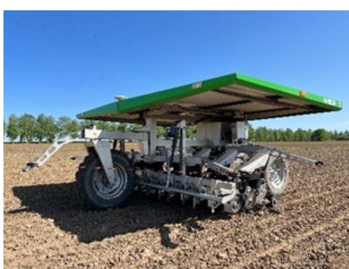
An autonomous solar-powered robot for direct seeding of sugar beet and mechanical weed control used for experiments in Lithuania.
