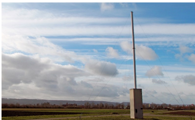
Stationary suction trap for long term monitoring at JKI in Quedlinburg/Harz (© T.Will, JKI)
